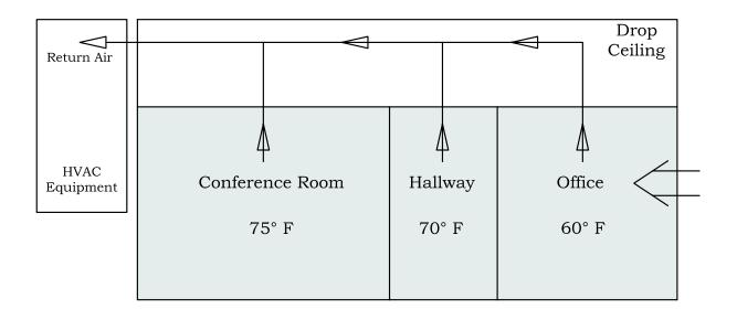
As shown above, this office is always colder than the other areas in the building and since the HVAC system is only supplying air that is a mixture of the 3 rooms shown, the office will continue to be colder although the employee in this office would like to keep the room at 75° F rather than the colder 60° F. What could be done to eliminate this problem?
