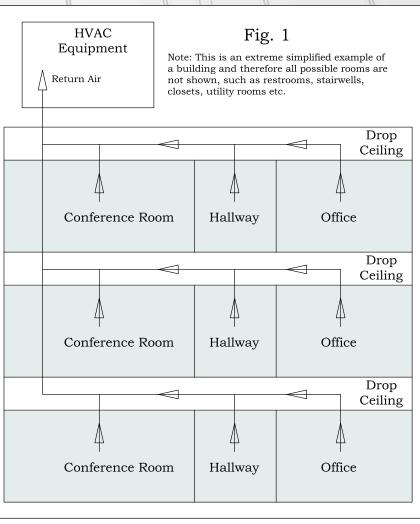
being used to gather air from required building spaces. This could indicate that the main HVAC system is responsible for gathering and mixing air at different temperatures and then conditioning this air to some pre-determined set values.
