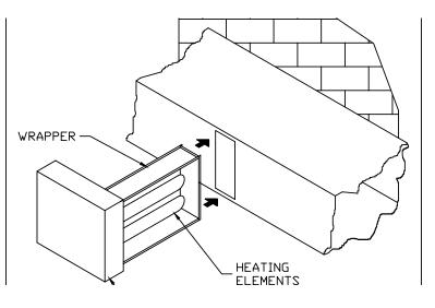
hole is cut in the duct, from one side only and the heater section containing the heating elements simply slides into the hole and the control box is sealed and fastened to the duct.
